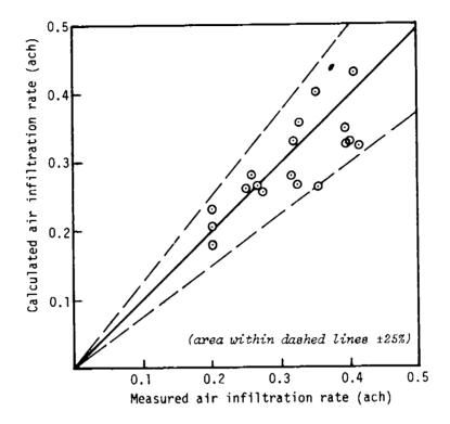
Figure 4.10.2: Comparison between calculated and measured air infiltration rates (HUDAC 'upgraded' house) (Reeves model)
