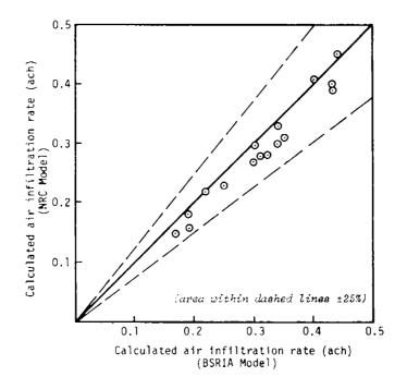
Figure 4.2.5: Comparison between calculated and measured air infiltration rates using NRC pressure coefficients (Maugwil house) (NRC model)
