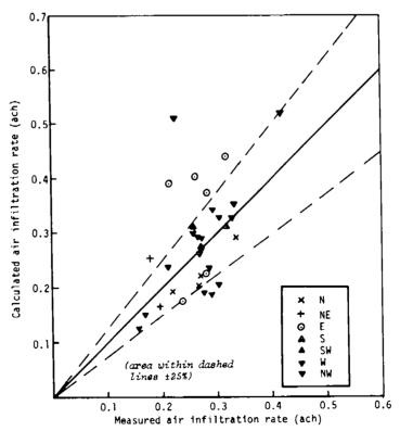
Figure 4.9.3: Comparison between calculated and measured air infiltration rates (HUDAC 'upgraded' house) (*BRE model*)
