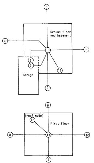
Figure 4.1.3: Node network (HUDAC Mk XI test house) (BSRIA model)
