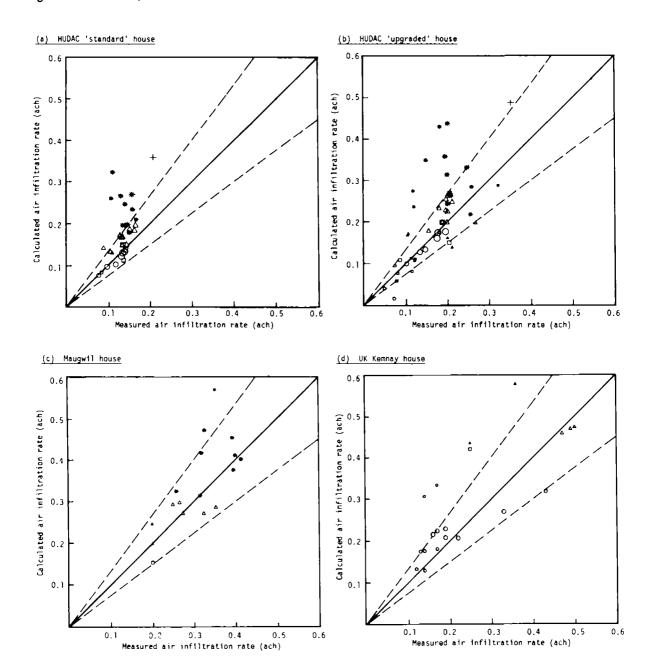
Figure 4.6.1: Comparison between calculated and measured air infiltration rates (NBRI model)
