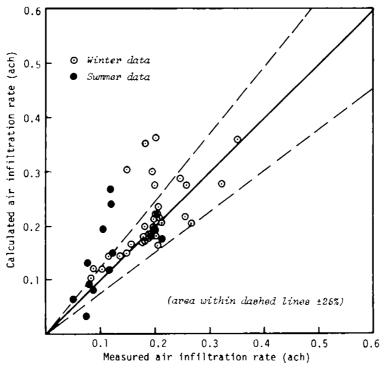
Figure 4.7.3: Comparison between calculated and measured air infiltration rates (Runcorn house) (IGT model)
