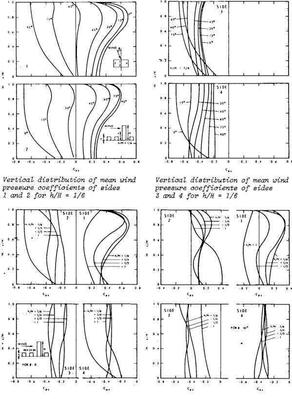
Vertical distribution of mean wind pressure coefficients for  $\theta = 0^{\circ}$  and various values of h/H
