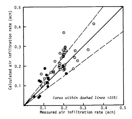
Figure 4.10.3: Comparison between calculated and measured air infiltration rates (Runcorn house) (Reeves model)
