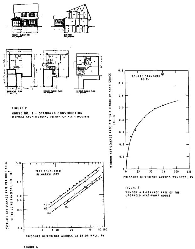
OVER-ALL AIR-LEAKAGE RATE FOR THE FOUR ENERGY-CONSERVATION RESEARCH HOUSES
